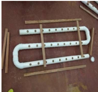
c) The PVCs and the base wood stand support cut using the vertical saw machine and assembled together using nails and hammer.
