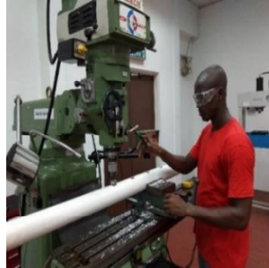
b) Drilling 45 mm diameter holes for placement of net pots, using the milling machine.
