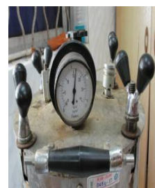
Sterilisation of ingredients in autoclave at 6.80 kg pressure
