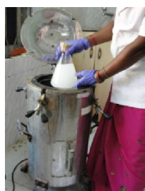
Placing conical flask in autoclave
